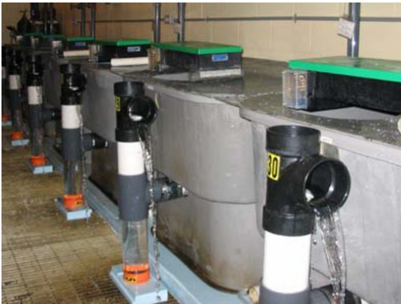
Figure 1: Rearing tank set-up with overflow and fecal collection vessels.
