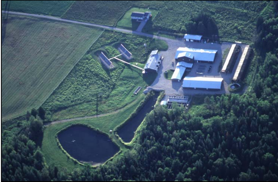
Aerial view showing polishing ponds for removal of fine settleable solids and adjacent property for land application of collected solids (liquid manure).
