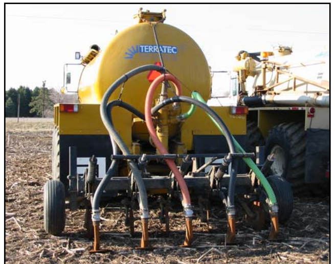
Liquid manure is land applied using a vacuum sprayer or injected into the soil.
